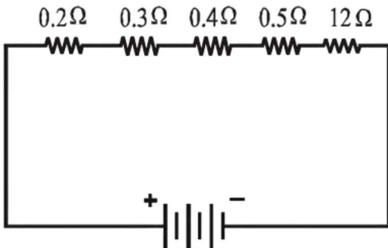
Since, The resistances are connected in series. Therefore, the value of current through each resistance will be same.
