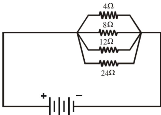
$$\frac{1}{R} = \frac{1}{R_1} + \frac{1}{R_2} + \frac{1}{R_3} + \frac{1}{R_4}$$
