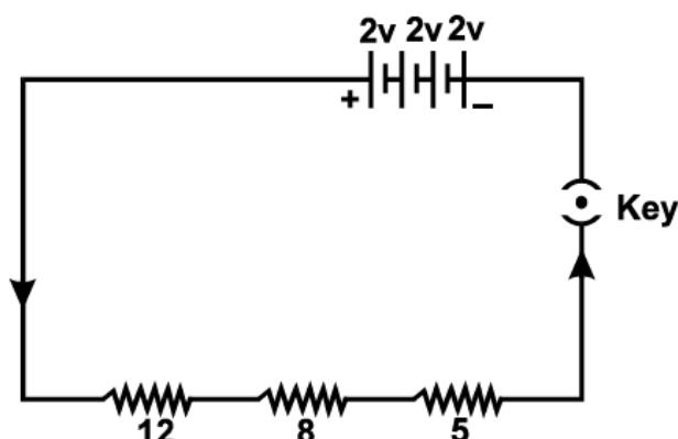
**Q13.** Redraw the circuit of above question, putting in an ammeter to measure the current through the resistor and a voltmeter to measure the potential difference across the 12 ohm resistor. What would be the readings in the ammeter and the voltmeter?
