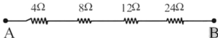
$$R = R_1 + R_2 + R_3 + R_4$$
