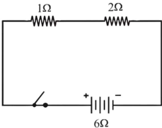
Current,  $I$  will be same in both resistors because they are connected in series.
